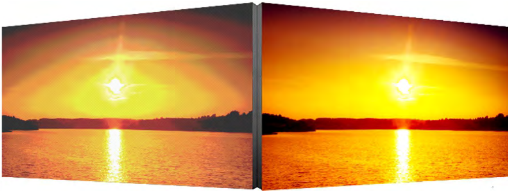
Figure 1: Comparing 8-bit (left side) vs. 10-bit image (on the right) shows the color banding effect
