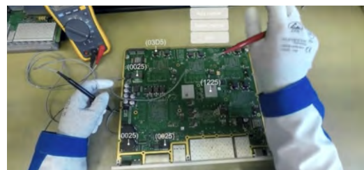
A technician repairs a circuit board using an augmented reality overlay at Ericsson's Tallinn factory. (Source: Ericsson)
