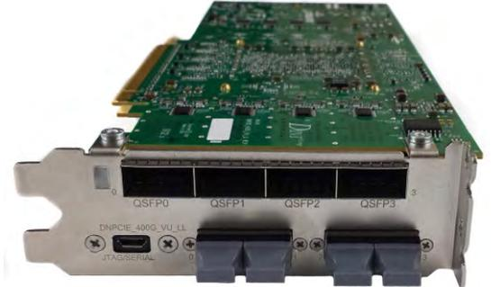
Five possible UltraScale+ FPGAs can be stuffed with the largest device, the VU13P, containing 20M ASIC gates with more than 12k, 27x18 multipliers. Five Virtex UltraScale and two Kintex UltraScale devices round out the possible FPGA stuffing options.
